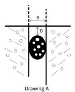
Materials used as backer rod should be weaker that the sealant itself and not obstruct the movement of the sealant whilst compressing or extracting.
